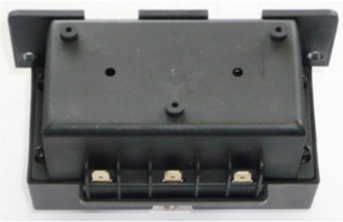
Open solenoid, remove the 4 screws in corner.
