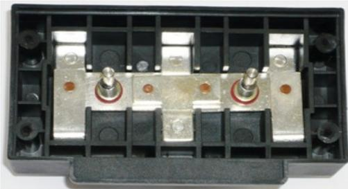
If contact plates are burned or corroded, clean with fine sand paper.
